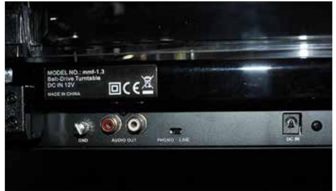
The rear panel sports the 12V DC input socket (plugpack supplied), a "GND" terminal and stereo RCA output sockets. You can choose RIAA line-level or "straight" phono output via the switch alongside the output sockets.
