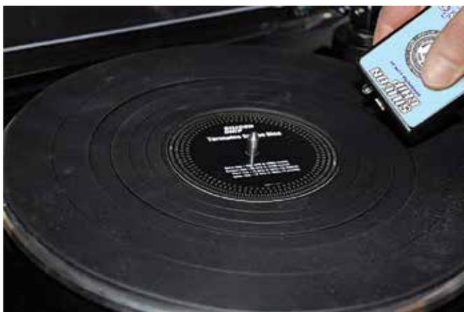
On unpacking the mmf-1.3 turntable, we checked the speed of the turntable with the SILICON CHIP strobe disc and white LED strobe (December 2015) and found it was spot on at all speeds, straight out of the box. . .
