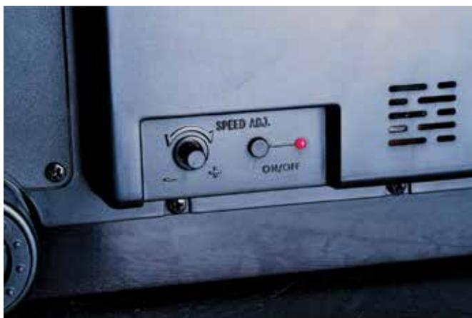
. . . but if it proved to be slightly “out”, it’s a simple matter of adjusting the speed by holding down the push button for two seconds then turning the knob. Unfortunately, it is under the turntable so takes a bit of juggling to get to!
