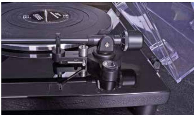
Here's the adjustment end of the tone arm, with the tracking dial at the rear and the anti-skate control closest to the camera. The tone arm is raised and lowered by the lever in the foreground.
